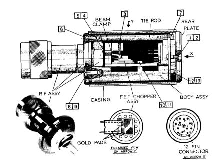
Fig. 5-1 Access and layout diagram - 6910 and 6930 Series Sensors
