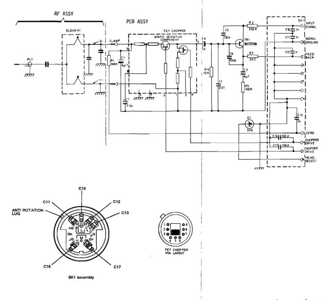
Fig. 7-1 Circuit diagram and component layout: 6913
