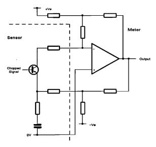
Fig. 4-2 Simplified Diagram of Amplifier
