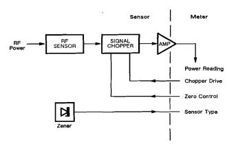
Fig. 4-1 Block Diagram of RF Power Sensor
