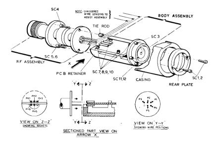
Fig. 5-2 Access and Layout Diagram - 6920 Sensor
